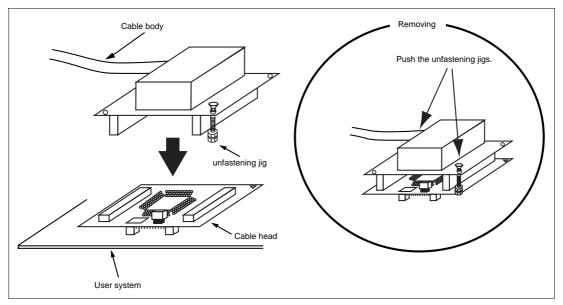
Figure 4 Fastening Cable Body
